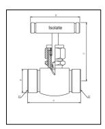
. HAVI Forged Needle Valve series has a Forged Body with Integral as well as Screwed Bonnet design with PTFE and Graphoil packing
